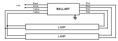
Ballast must be grounded. Install in accordance with National Electric Code.
