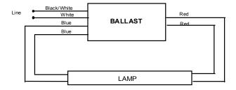
Ballast must be grounded. Install in accordance with National Electric Code.
