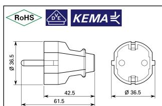
515ZL Power Supply Cord (2-Pole 3-Wire Grounding) with attached Plug No. 515 (not rewireable) (CEE 7/4)
