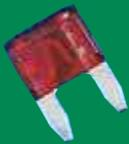
The MINI fuse is smaller than its predecessor, the ATO fuse, which permits using more fuses in the same amount of space. More fuses in the same space satisfies the requirement that more circuits be individually fused in newer automobiles. Patented by Littelfuse.
