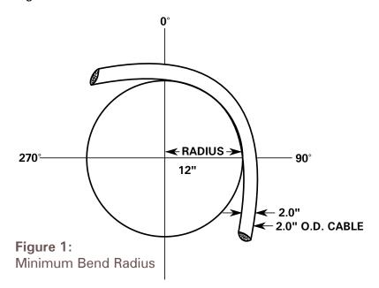
The minimum bend radius is based on the diameter of the cable and the type of cable. The following formula is used:
